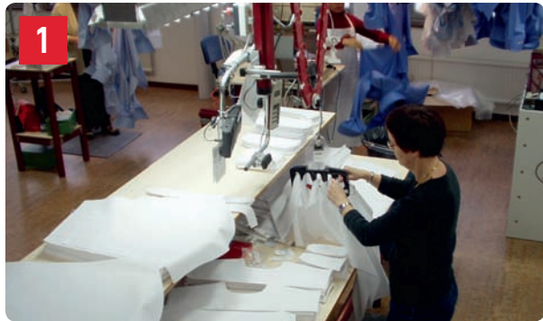
1 Loading of pieces for one complete unit in the product carrier.
