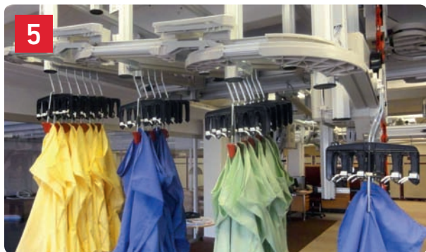
5 Multi-rail stations can automatically both sort and buffer products within a workstation. This maximizes operator productivity.
