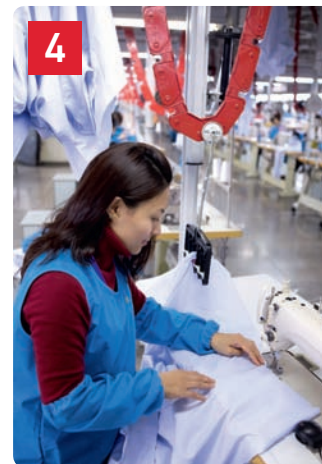
4 The Eton Systems workstation delivers greater operational efficiency and ergonomics, as most operations can be performed without removing the garment from the carrier.
