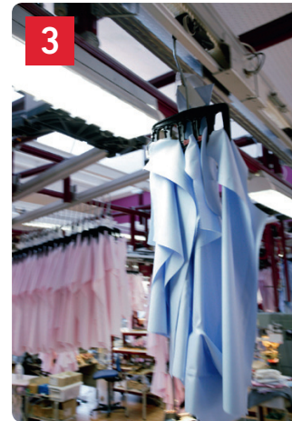
3 All pieces for one unit have specific positions in the product carrier. The product carriers are transported between workstations on the main line.
