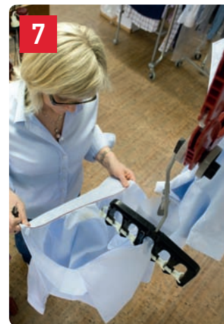
7 Inspection stations. The Eton Systems chain allows for both sitting and standing configurations.
