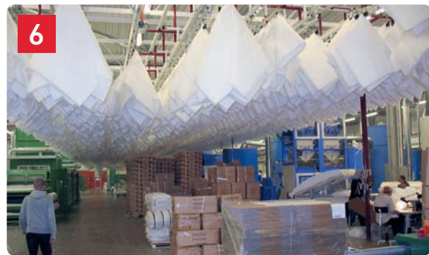
Overhead feeding buffer for optimal utilization of space.
