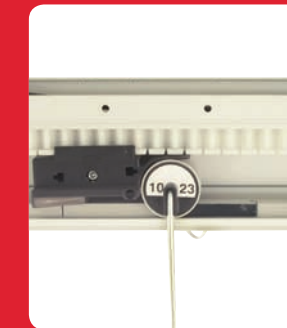
Automatic routing and tracking throughout the process. Each product carrier has a unique identity.
