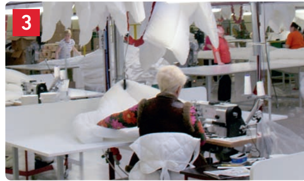
High efficiency thanks to the chain. Most of the operations can be performed without removing the product from the product carrier.
