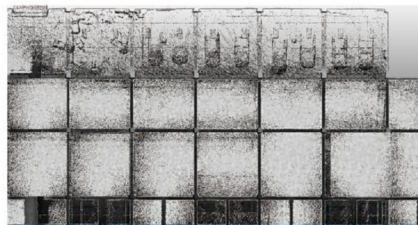
Rotating scanning making the top and bottom data uniform and the corner data complete
