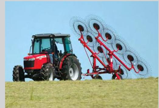
**ONE SINGLE-ACTING CYLINDER** folds both wings for easy transport (available on 1508, 1510 and 1512 models).
