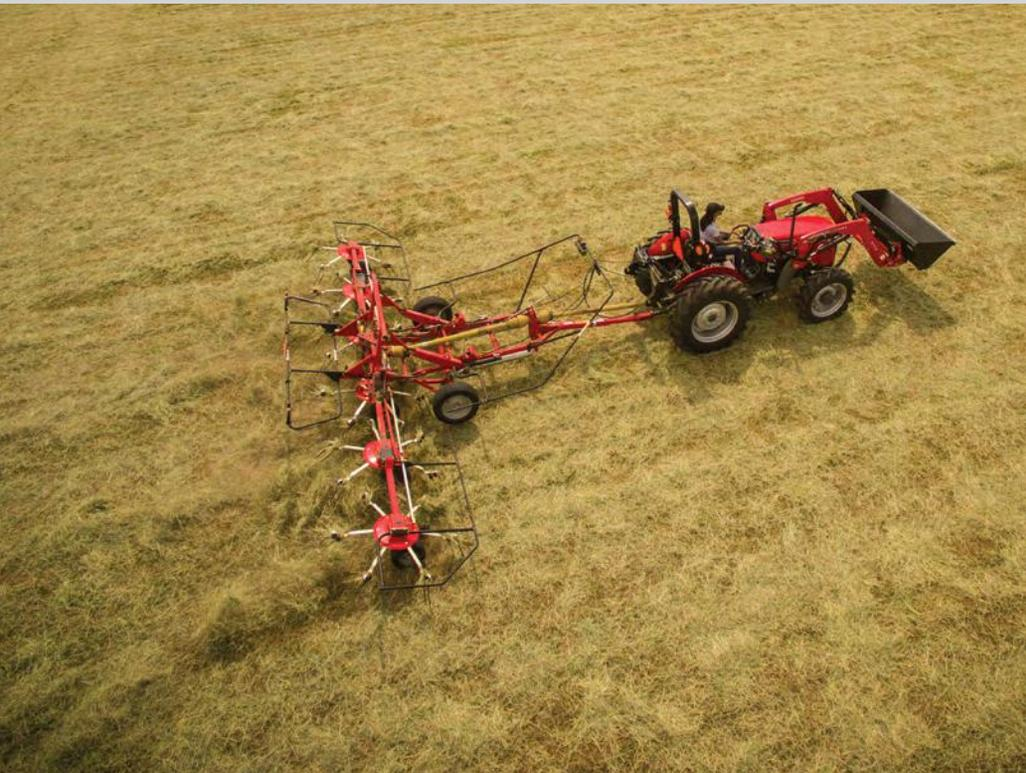
All models are simple to set-up and adjust for quick and efficient ground coverage. Four, six, eight and 10-rotor models also feature synchronized lifting of exterior rotors via a centralized hydraulic lift system and pressure cylinders to ensure optimum performance and eliminate one-sided loads — even on slopes.
