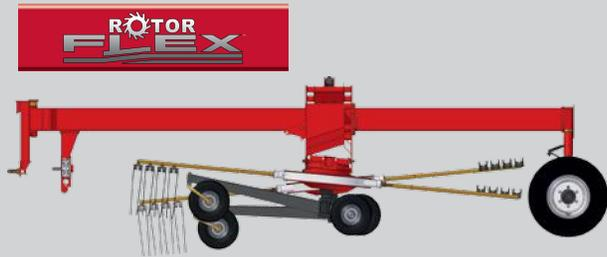
**THE ROTORFLEX SUSPENSION** features “jet-effect” lifting and lowering, which means the front lifts first and lowers last, to keep tines from diving into the ground.
