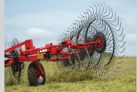
**ADJUSTABLE FLOAT SPRINGS** on each rake arm let the operator select just the right amount of down pressure for the crop and field conditions.
