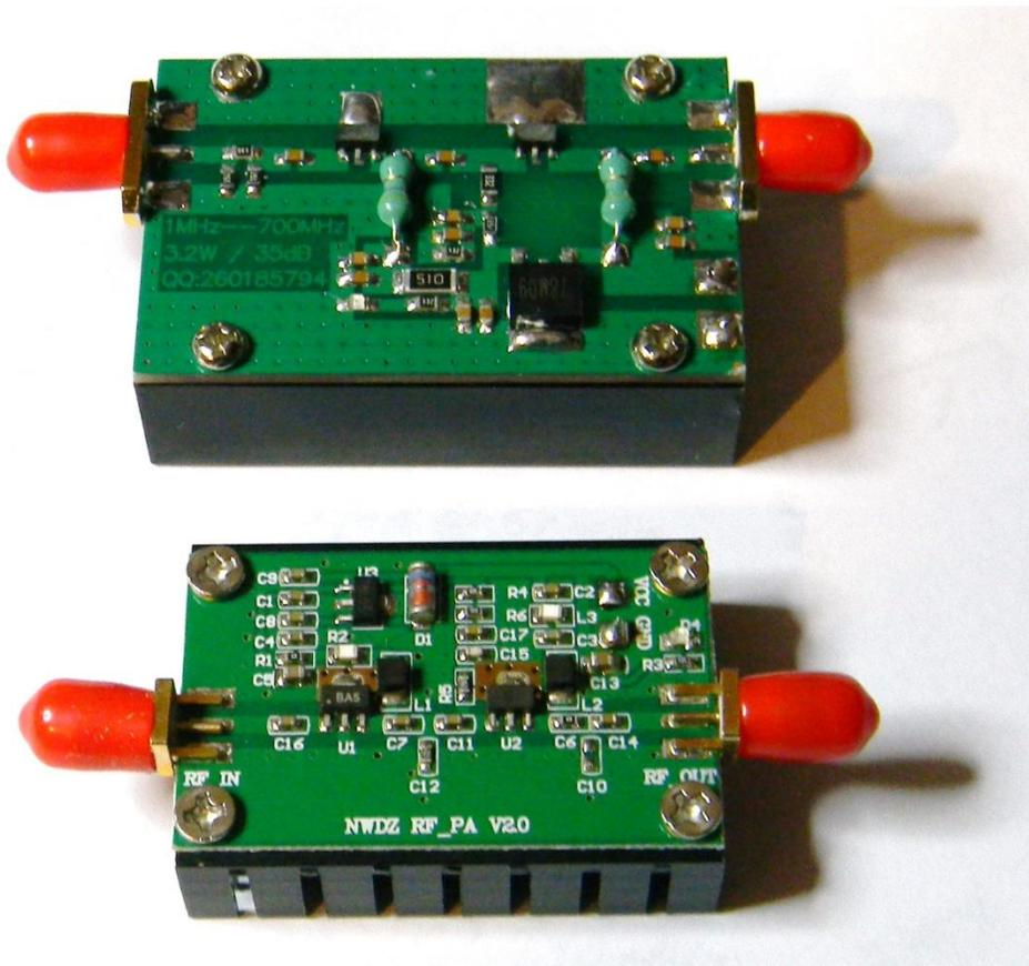
**Two different final amplifiers suitable for use with this transceiver. Either will put out 1-3 watts.**
