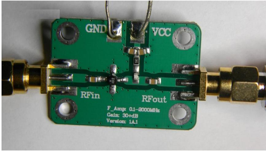
**Recommended Buffer Amplifier. It may be necessary to construct a shield over this side if unwanted RF is coupled to other components or wiring. Construct from copper or tin and ground to connectors at each end and unused mounting holes. Avoid VCC.**
