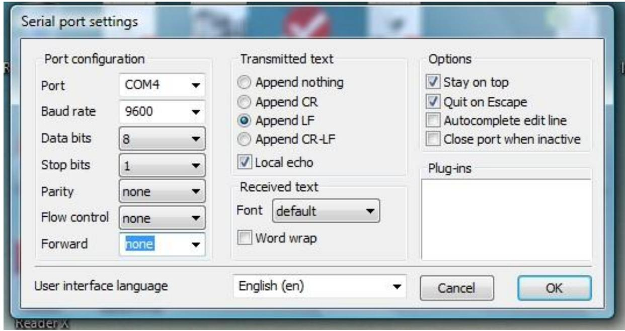
**Figure 2 Serial control software, Port may change for your computer**
