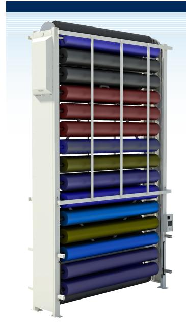
The Multi-Roll Carousel system, available in many sizes and styles, provides tremendously simple access to multiple material rolls for end-of-table spreading, using minimal floor space. With the press of a button, material rolls turn around the carousel, stopping on the desired roll.
