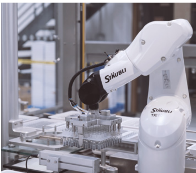
Dedicated grippers are used for handling the tubs.
