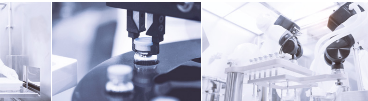
A robotic arm prepares to place a finished vial back into the nest.
