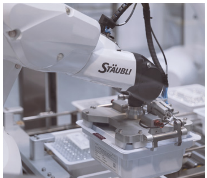
The third robot covers the tubs with a lid and applies two labels.
