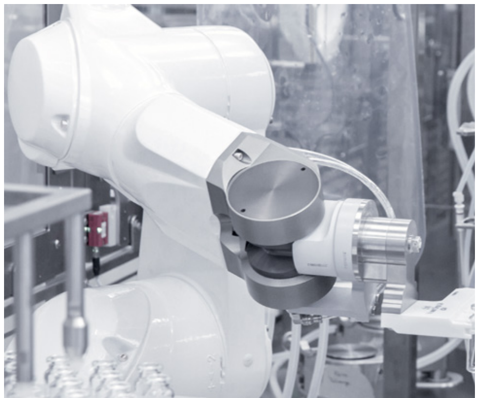
The smooth surface of the Stericlean robots are easy to clean and meet the hygiene requirements of the pharmaceutical industry.
