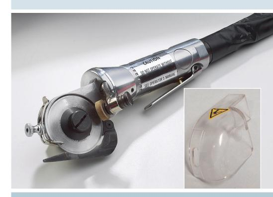
The Buzzaird® is designed with a 20,000 RPM pneumatic motor suitable for wet environments. It is an extremely powerful rotary shear suitable for cutting single-ply leather, rubber, plastics, woven glass, coated materials, and much more. Available options include a Pelican head or swivel sharpener. Optional swivel sharpener is equipped with a 30 degree ball tip shear plate for close edge trimming.
