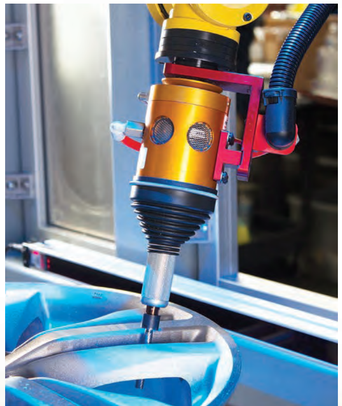
ATI RC-300 Deburring Tool utilized in automotive wheel deburring.
