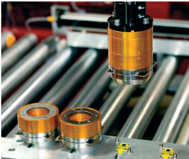
Custom Tool Changer developed for automated box opening system.
