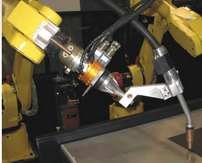
QC-20 Robotic Tool Changer utilized to exchange welding torches.
