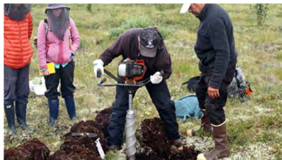
Figure 33. Sasha powering into the permafrost with the Cipre corer.
